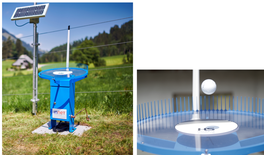
Figure 2. Left: Picture of one of the automatic hail sensors installed in the project "Swiss Hail Network" (© Manu Friederich). Right: Zoom on the sensor Makrolon disc as a golf ball is falling (La Mobilière / Sascha Moetsch)
