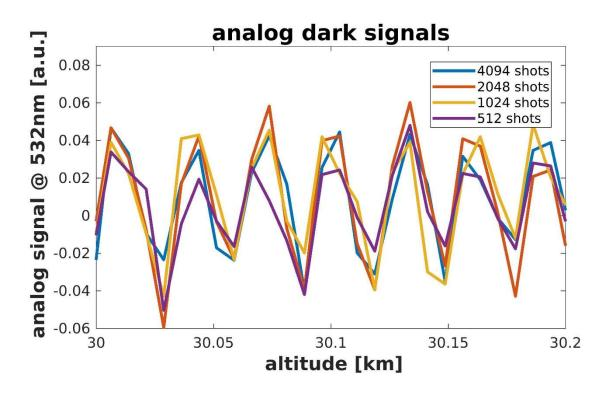
If the strength relative to the lidar signal does not change with averaging, the interference signal must be in phase with the laser repetition.
