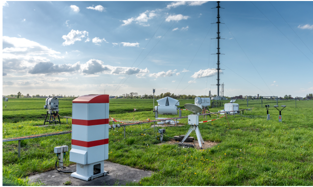
Figure 2. The ceilometer (in front) and 213-meter mast (background) at the same location at Cabauw support high-quality annotations. This site also includes a scanning microwave radiometer (left), a scanning cloud radar, a micro rain radar and a second microwave radiometer (center), a scanning Doppler wind lidar and two distrometers (right).
