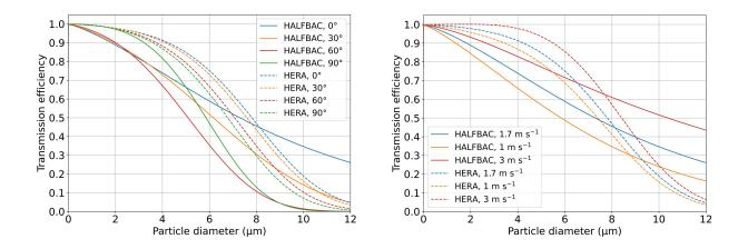
The left plot shows the sampling efficiency at a constant wind speed of 1.7 m/s (same as mean wind speed during sampling periods 4 and 5) with variable aspiration angle of 0° (inlet facing wind directly) to 90° (inlet facing wind at 90°). Solid lines represent HALFBAC ( $\frac{1}{2}$  inch inlet), dashed lines HERA ( $\frac{3}{4}$  inch inlet). The right plot shows the sampling efficiency at a
