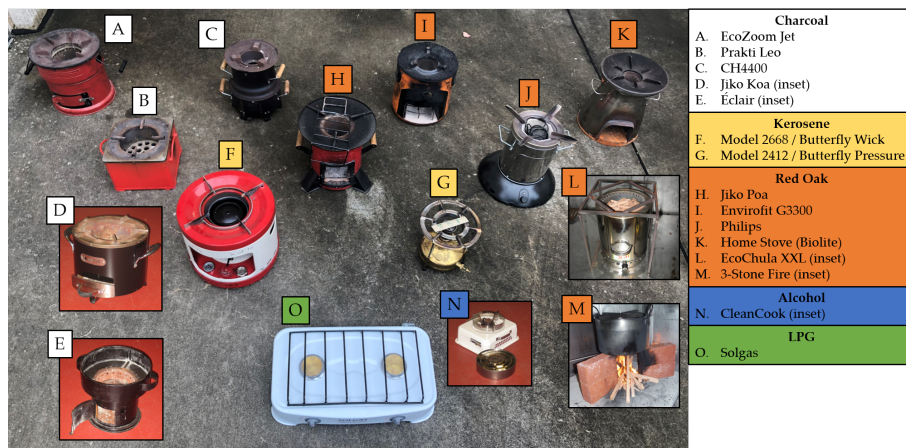
Figure 2. Photo showing 15 stoves used in this work. Charcoal stoves: (A) EcoZoom Jet, (B) Prakti Leo, (C) Envirofit CH4400, (D) Jiko Koa (inset), and (E) Éclair (inset). Kerosene stoves: (F) Model 2668 / Butterfly Wick and (G) Model 2412 / Butterfly Pressure. Red oak wood stoves: (H) Jiko Poa, (I) Envirofit G3300, (J) Philips HD4012, (K) Home Stove (Biolite), (L) EcoChula XXL (inset), and (M) 3-Stone Fire (inset). Alcohol stove: (N) CleanCook (inset). LPG stove: (O) Solgas.
