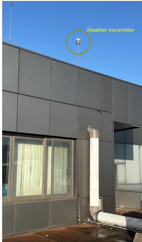
Figure 2. Installation of the weather sensor (WXT510) on the roof of the building
