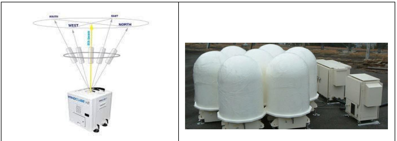
Figure 1: (Left) The WindCube v2 Infrared Doppler Lidar, manufactured by Leosphere and provided by EKO Instruments Co., Ltd. (Japan) along with the 5 beam directions. (Right) The WPR LQ7 antenna array.
