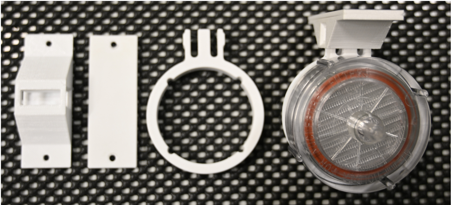
Figure 2: 3D printed parts for the filter holder mounting to the plane. From left to right: mount base, mount backplate, filter holder mount and final setup . The mount base is connected to the wing by the backplate, while the filter holder snaps into the base and secures the position of the filter holder.
