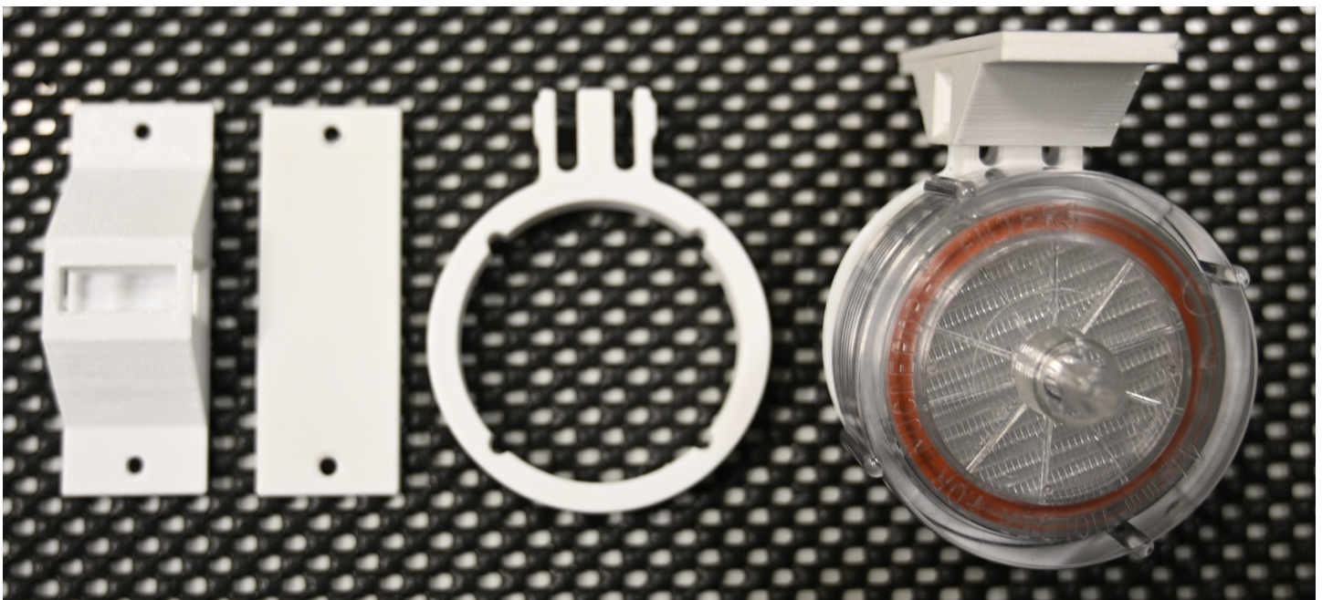
Figure 3: 3D printed parts for the filter holder mounting to the plane. From left to right: filter holder mount , mount base , mount backplate . The mount base is connected to the wing by the backplate, while the filter holder snaps into the base and secures the position of the filter holder.
