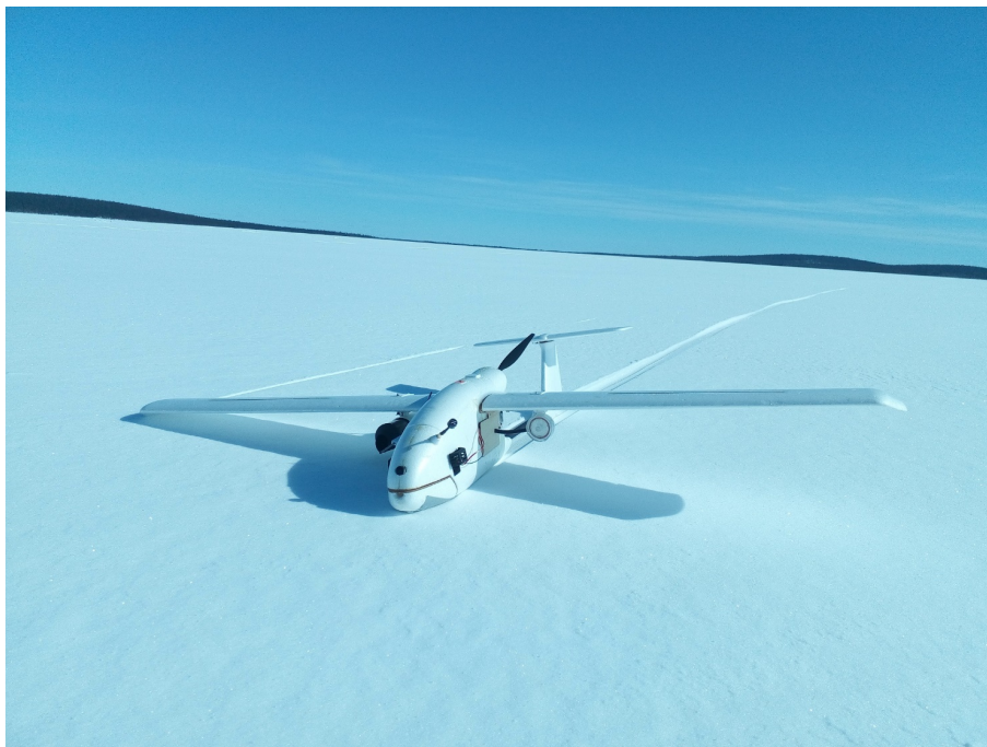
Figure 1. The Skywalker shown with the final setup after a successful flight. The filter holder is installed with a tube connection through the wooden side plate. The inlet is blocked until launch. On the right, the ambient sensor (BME280, Bosch) can be seen, and the airspeed sensor is visible on the left side ( ASPD-7002 ASPD-7002 , Matek Systems).
