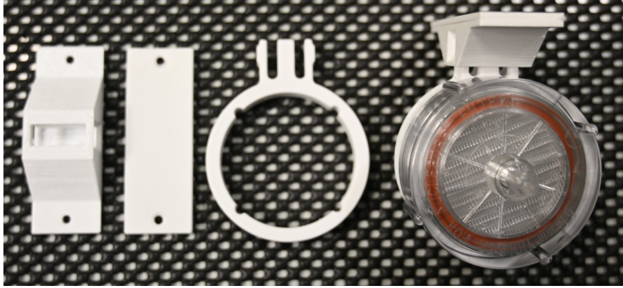
Figure 2. 3D printed parts for the filter holder mounting to the plane. From left to right: filter holder mount , mount base , mount backplate , filter holder mount and final setup . The mount base is connected to the wing by the backplate, while the filter holder snaps into the base and secures the position of the filter holder.
