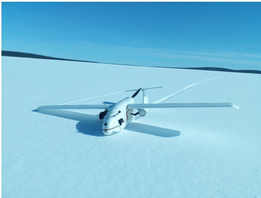
Figure 1. The Skywalker shown with the final setup after a successful flight. The filter holder is installed with a tube connection through the wooden side plate. The inlet is blocked until launch. On the right, the ambient sensor (BME280, Bosch) can be seen, and the airspeed sensor is visible on the left side (ASPD-7002, Matek Systems).
