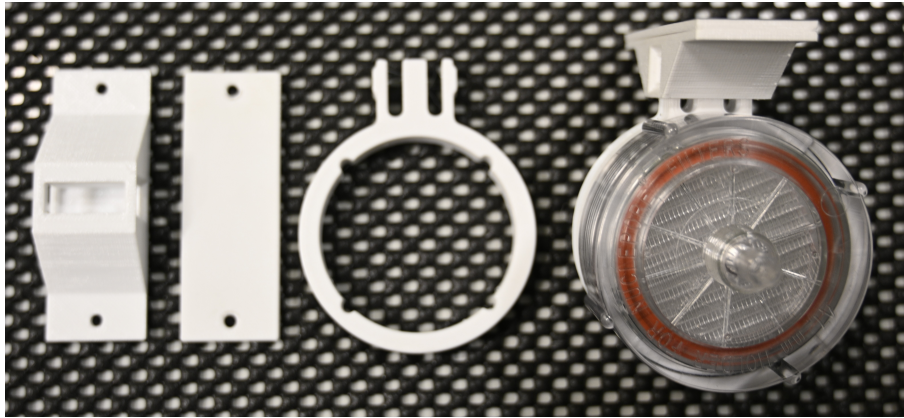
Figure 2. 3D printed parts for the filter holder mounting to the plane. From left to right: mount base, mount backplate, filter holder mount and final setup. The mount base is connected to the wing by the backplate, while the filter holder snaps into the base and secures the position of the filter holder.
