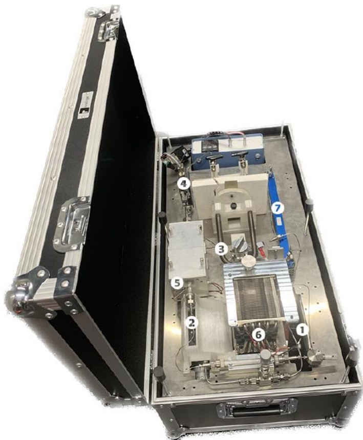
85 Figure 2: Setup of the atmospheric methane sampling device. The whole system fits well into a box of 80 x 40 x 30 cm. It runs either on 115/230 V AC or 48 V DC provided by a battery pack. Major parts of the system are: 1) Nafion dryer (mostly hidden underneath); 2) Pumps (partially hidden); 3) CO 2 trap; 4) Flow controller; 5) Furnace for CH 4 combustion; 6) Sample trap with Peltier coolers; 7) CO 2 sensor
