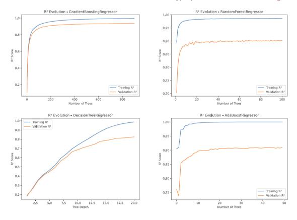
We can observe in the above plots during the different iterations the fit of the model in terms of R<sup>2</sup>, with a better fit with training than with validation, as expected. In addition, it should be noted that the convergence process with training does not reach a perfect fit in any case, which justifies and supports the conclusion that there is no overfitting in the models.
