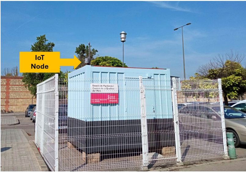
Figure 1. Detail of the standardized AQ monitoring station and the AQ node with a ZPHS01B module located at Bulevar Sur (Valencia, Spain).
