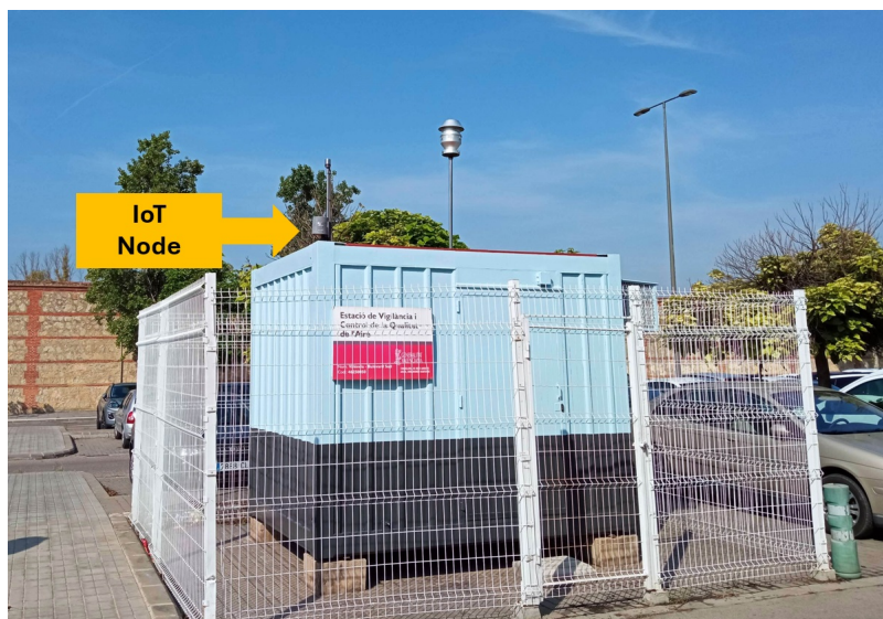
Figure 1. Detail of the official AQ monitoring station and the AQ node with a ZPHS01B module located at Bulevar Sur (Valencia, Spain).
