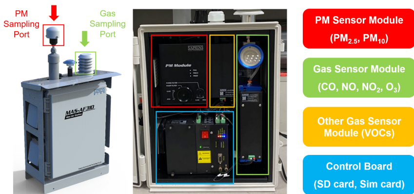
Figure 1. Structure diagram of MAS monitoring devices (dimensions: 420 × 320 × 180 mm, H × W × D; weight: 12 kg; power consumption: 15W).
