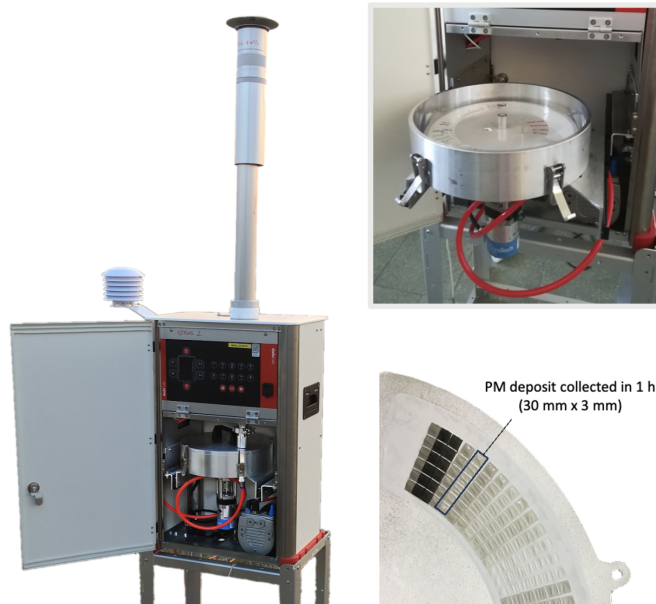
Figure 1: The STRAS sampler. On the left, a picture of the whole sampler: the chamber with the rotating system can be seen inside the cabinet. On the right, a picture of the chamber when it is extracted (using linear guides) to be opened for inspecting or changing the filter. Below, a picture of a portion of the collecting polycarbonate membrane, where aerosol deposits can be seen.
