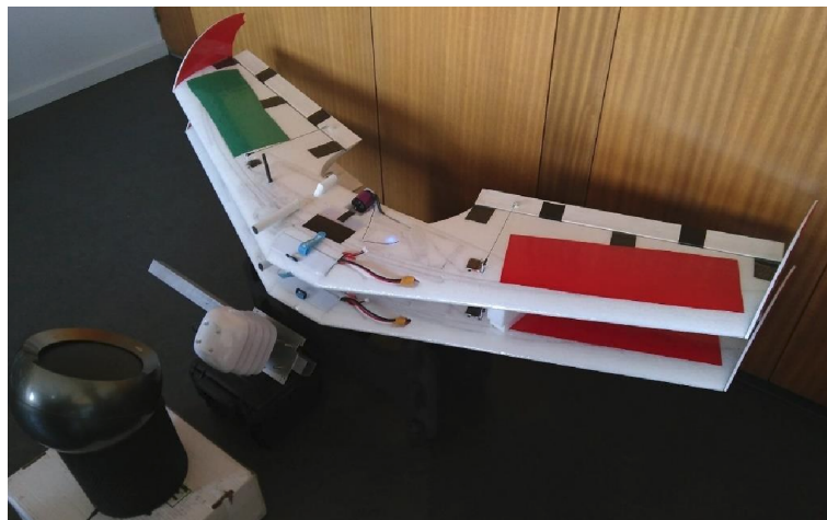
Figure A1. Setup of the 24-hour intercomparison measurement of the temperature and humidity sensors (SHT75) installed inside the white tube of each UAV and a reference sensor (SHT21, inside the radiation shield) placed in front of both UAVs. A fan ensured continuous air flow. The experiment was conducted from 4 to 5 June 2021.
