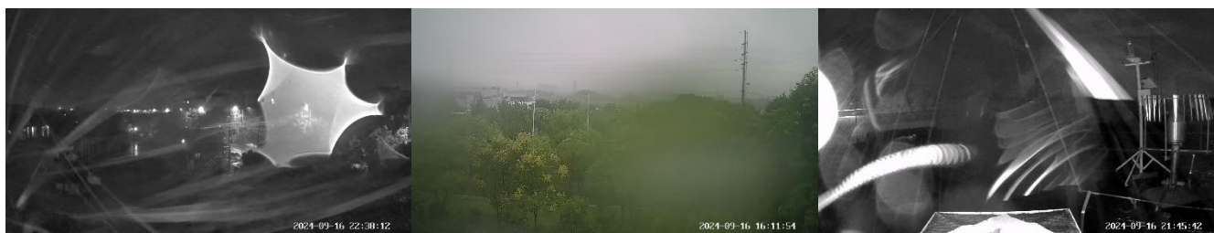
645 (a) Drop attachment on lens at night (b) Daytime drop attachment on lens (c) Wind caused image blurred
