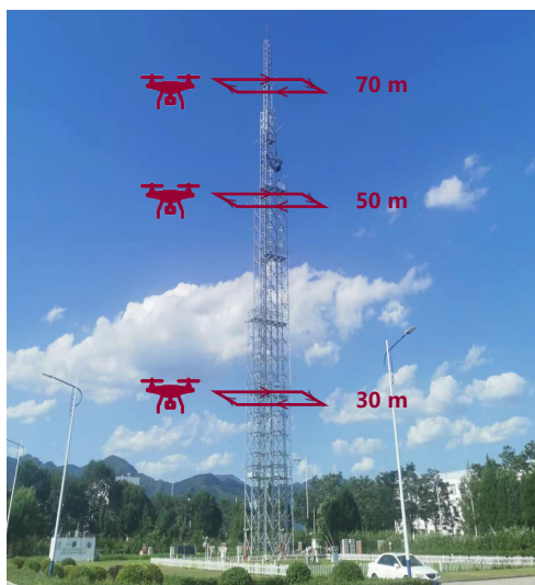
397 398 Figure 8: Comparative experiment on wind measurements between the UAV and the meteorological tower.
