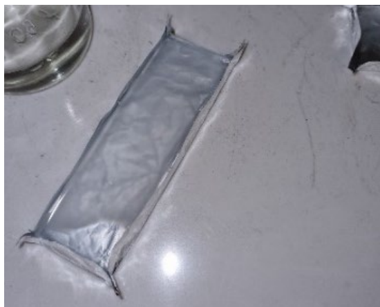
Figure 1. Aluminium foil container with formvar solution pool.
