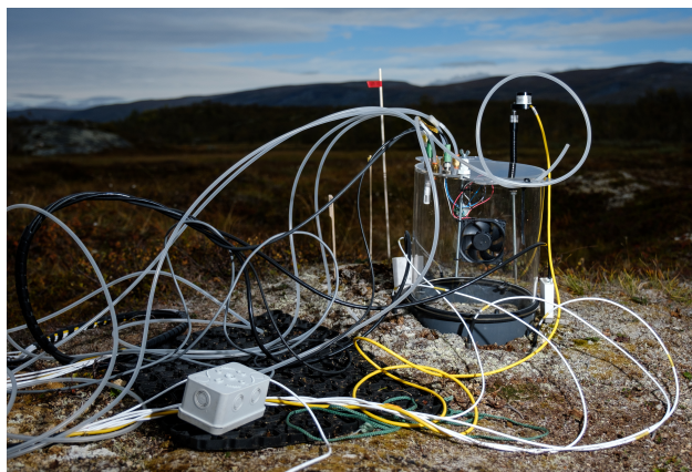
Figure 2. Chamber setup during measurement period, with soil moisture and soil temperature sensors installed in the soil, and all inlets connected. Photo: Fabio Cian, “Ubiquitous Anomaly”, CC BY-NC-ND 4.0
