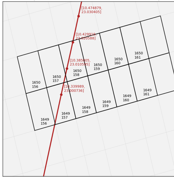
Figure A1. TROPOMI ground pixels at BD3 grid (black color) and CALIPSO overpass measurements (red color). One or even two CALIPSO data points can fall into the TROPOMI BD3 ground pixel. Every TROPOMI ground pixel contains two numbers; the first refers to the scanline and the second to the pixel id. The CALIPSO measurements are identified directly with the geographic coordinates.
