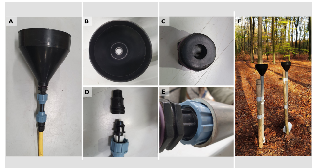
Figure 2. Construction of the deposition samplers. A: the connected sampler ready for use in the field. B: the used funnel with a collection surface of 288 cm 2 . C: the wire coupling between the funnel and the resin column containing a mesh to prevent larger objects entering the resin column. D: overview of the resin column with the wire couplings. E: the resin column fitted tightly into the PVC tube, which allowed easy installation of the resin columns in the field. F: paired samplers in the field.
