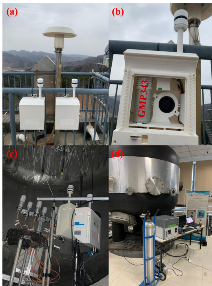
122 Fig. 1. The internal structure of Luccn and the observation field diagrams in the laboratory. (a) is the exterior 123 diagram of Luccn ground stations, and (b) shows the internal composition of Luccn. (c) shows the NDIR 124 sensors and gas conduits placed inside a cloud chamber where temperature, pressure and humidity can be adjusted 125 according to demands. (d) shows the exterior of cloud chamber, Picarro G2301 and WMO CO 2 standard gas 126 cylinders.
