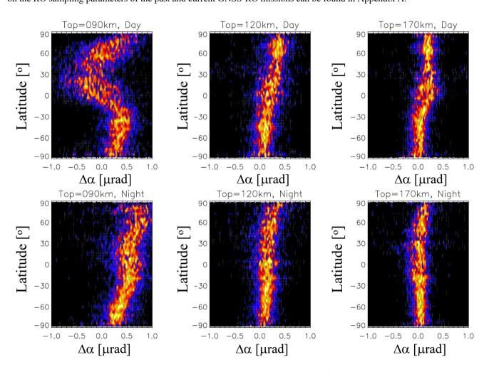
Fig.16. Probability distribution function (PDF) of the RIE derived from the  $-d\phi_{ex}/dh_t$  algorithm to compare impacts of the RO top height truncation. The experimental data from the MetOp-A special scan during D161-D254 in 2020 were used in the analysis and the RIE statistics from day (top panels) and night (bottom panels) are reported separately. The RIE results from three RO cutoff top heights, 90, 120, and 170 km, are selected for comparisons.
