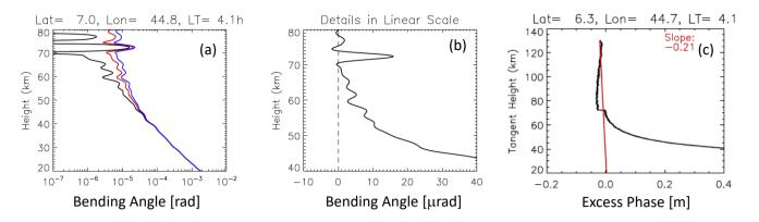
170 Fig.3. As in Fig.1 but for a case with a sharp jump in the  $\phi_{ex}$  profile near 70 km and a moderate derivative  $d\phi_{ex}/dh_t$ .
