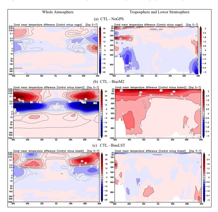
Fig.15. The zonal mean temperature differences between controlled and perturbed experiments. A different color scale is used for the lower atmosphere, to highlight small values in this region.
