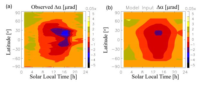
Fig.14. (a) Annual mean  $\Delta \alpha$  variations derived from 2013 COSMIC-1 data; (b) Parameterized  $\Delta \alpha$  variations used as the RIE input for the "BiasLST" DA experiment. All color numbers have a scale factor indicated at the top of each colorbar.
