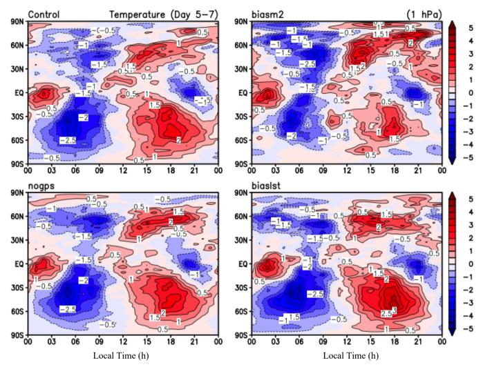
670 Fig.B1. Diurnal temperature variations from the controlled and perturbed experiments at 1 hPa. The temperature perturbations from its zonal mean in K are contoured in color.
