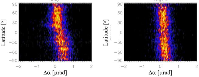
Fig.5 Latitude dependence of the probability density function (PDF) of COMSIC-1  $\Delta \alpha$  in µrad for day and night from Jan 2013. The PDF is normalized independently to its peak value at each 4° latitude bin. The PDF colors vary linearly between 0 (black) and 1 (yellow).
