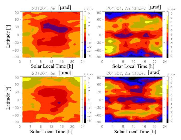
**Fig.10.** Latitude (4°-bin) and solar local time (2h-bin) dependence of COSMIC-1 RIE  $\Delta \alpha$  mean (μ) and standard deviation (σ) from January and July 2013. All color numbers have a scale factor indicated at the top of each colorbar.
