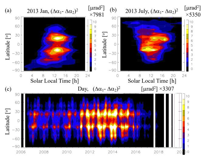
Fig.12. The  $(\Delta \alpha_1 - \Delta \alpha_2)^2$  distribution and variations derived from the COSMIC-1 data using  $\Delta \alpha_1 \equiv -d\phi_{exL1}/dh_t$  and  $\Delta \alpha_2 \equiv -d\phi_{exL2}/dh_t$ . The  $(\Delta \alpha_1 - \Delta \alpha_2)^2$  distribution here can be compared to the RIE derived from the κ-method in Fig.10, by multiplying a κ value between -10 and -15 rad<sup>-1</sup> for 60 km. All color numbers have a scale factor indicated at the top of each colorbar.
