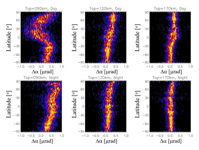
Fig.16. Probability distribution function (PDF) of the RIE derived from the  $-d\phi_{ex}/dh_t$  algorithm to compare impacts of the RO top height truncation. The experimental data from the MetOp-A special scan during D161-D254 in 2020 were used in the analysis and the RIE statistics from day (top panels) and night (bottom panels) are reported separately. The RIE results from three RO cutoff top heights, 90, 120, and 170 km, are selected for comparisons.
