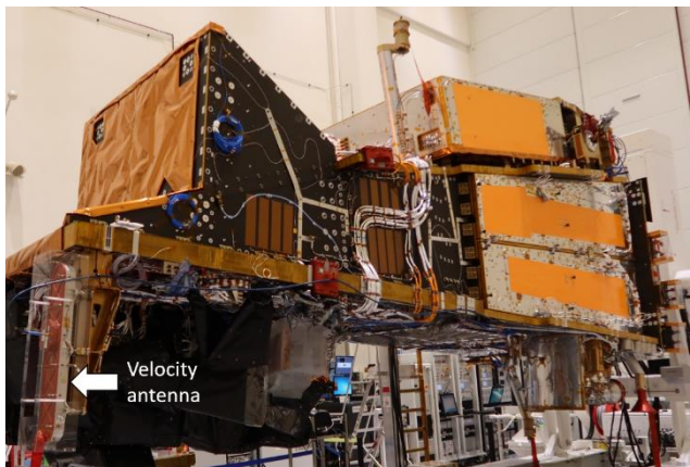
Figure 7: Proto-flight model satellite and RO units with test-caps to allow testing on satellite level. Source: Airbus Defence and Space SAS/ GmbH. Notes: MetOp-SG is a collaborative programme between ESA and EUMETSAT. Airbus Defence and Space is Prime contractor, under ESA, for the two Satellites series contracts. Picture shows satellite in assembly phase and not in its final configuration
