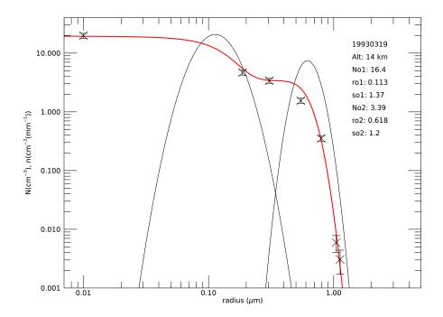
**Figure 3.** Example of WOPC measurements (black crosses). The black lines show the two modes fit during the processing of WOPC data. The cumulative bimodal log-normal distribution is shown in red. Error bars are shown accounting for the Poisson error.
