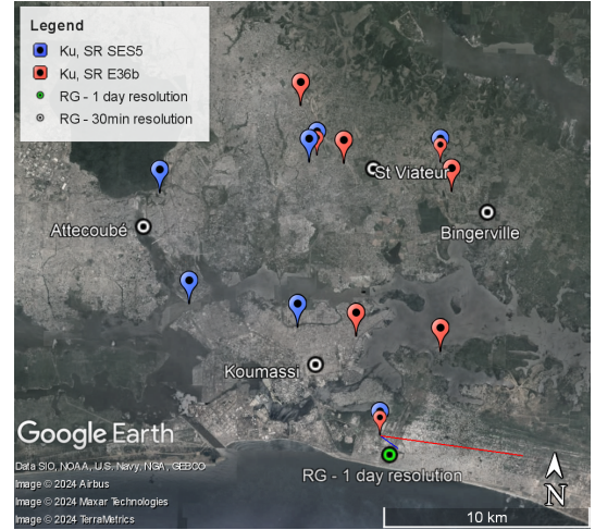
Figure 4. Map of available devices in the Abidjan area: Ku-sensors colored according to the satellite they target, E36b (red marker) and SES5 (blue marker); the link path is identified by coloured lines corresponding to the distance between the sensor and the 0°C isotherm (here taken to be 4500m) in the satellite target (for legibility reasons, only 2 paths have been drawn as examples); rain gauges represented by points with an enclosed circle: in white for the four 30-minute resolution rain gauges and in green for the Abidjan airport rain gauge at 1-day resolution (From Google Earth Pro).
