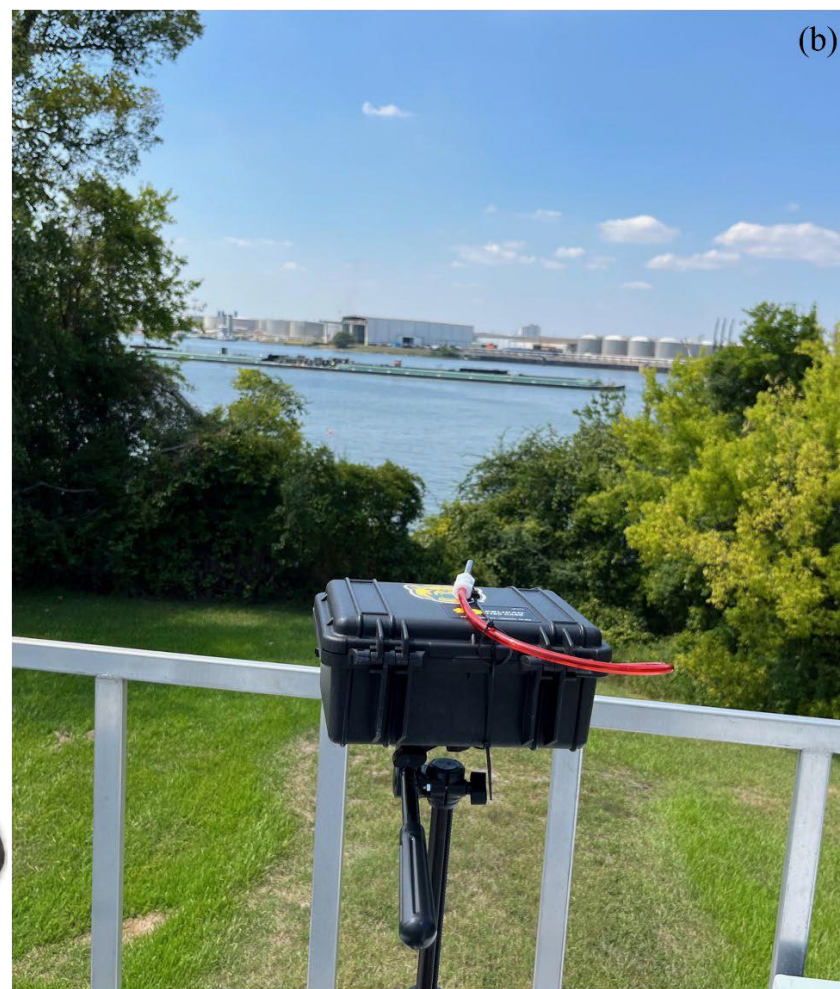
Figure S3. During TRACER-AQ2, a single tube sampler (a) with identical internal power and flow components as the aerial samplers described in this study was deployed in the field (b).
