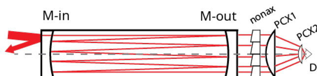
Figure 6. Schematic of the ChiWIS cell and detection optics with the NonAx component included. The NonAx optic is placed between the cavity output mirror and PCX1, where the output rays are nearly paraxial, and refracts out most of the skewness in those rays before they are focused down to the optical axis and onto the detector. Figure adapted from (Clouser et al., 2018).
